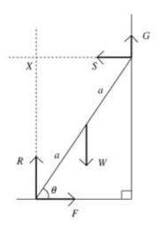
R and F are the normal reaction and the friction where the ladder is in contact with the ground. S and G are the normal reaction and the friction at the wall.
