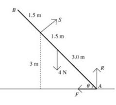
S is the normal reaction at C, R is the normal reaction at A, and F is the friction at A.  $\theta$  is the angle between the pole and the ground.
