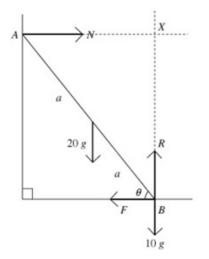
Let the ladder have length  $2\alpha$ , and be inclined at  $\theta$  to the horizontal.
