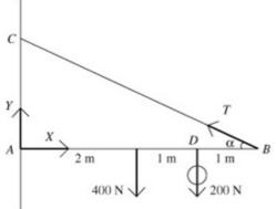
Let the tension in cable BC be T. The horizontal and vertical components of the tan  $\alpha = \frac{1}{2} \Rightarrow \sin \alpha = \frac{1}{\sqrt{5}}$ reaction at A are X and Y respectively.
