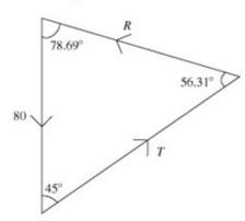
$\frac{R}{\sin 45^{\circ}} = \frac{T}{\sin 78.69^{\circ}} = \frac{80}{\sin 56.31^{\circ}}$   $R = \frac{80 \sin 45^{\circ}}{\sin 56.31^{\circ}} = 68.0 \text{ N at } 78.69^{\circ} \text{ to the}$ upward vertical and  $T = \frac{80 \sin 78.69^{\circ}}{\sin 56.31^{\circ}} = 94.3 \text{ N}$
