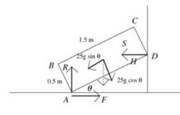
R and S are the normal reactions at A and D respectively. F is the friction at A.
