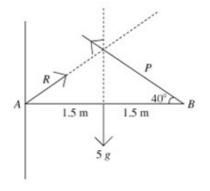
Because the rod is uniform we know that the centre of mass is at the mid-point of the rod. This implies a symmetrical diagram (isosceles triangle), so we know that R acts at  $40^{\circ}$  to the rod and the magnitudes of P and R are equal.
