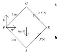
PQR is an isosceles triangle with two sides of 3 m, so the length of PR is  $3\sqrt{2}$  m.
