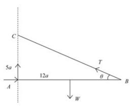
Let the angle between the string and the rod be  $\theta$ , T be the tension in the string, X the horizontal component of the force at A and Y the vertical component of the force at A.
