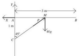
The lines of action of P and the weight meet at M, hence the line of action of the resultant of X and Y must also pass through M (3 forces acting on a body in equilibrium). Therefore the reaction must act horizontally (i.e. no vertical component).
