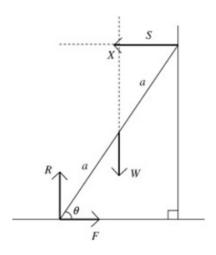
Suppose that the ladder has length 2aand weight W. S is the normal reaction at the wall, R is the normal reaction at the floor, and F is the friction at the floor. X is the point where the lines of action of W and S meet.
