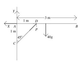
Let the horizontal and vertical components or the force at A be X and Y respectively. Let the thrust in the rod be P.
