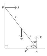
Let A and B be the ends of the ladder. S is the normal reaction at B, R the normal reaction at A and F the friction at B. The length of the ladder is 2a. а
