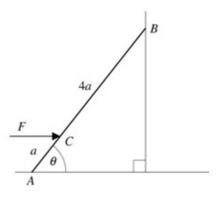
Let S be the force between the ladder and the wall at B. Let R be the normal reaction at A. (Both surfaces are smooth, so no friction.)
