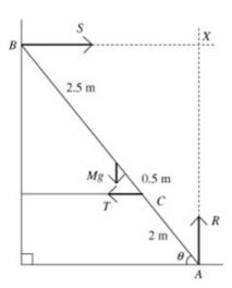
Given  $\tan \theta = 2$ . The normal reactions at A and B are R and Srespectively. X is the point where the times of action of R and S meet. T is the tension in the string.
