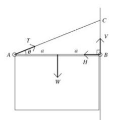
T is the tension in the string, V and H are horizontal and vertical components of the force at B.
