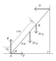
Suppose that the boy reaches the point B, distance x from A, the end of the ladder in contact with the ground.
